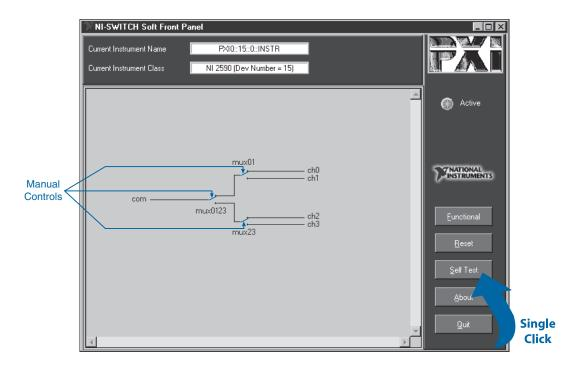
Run the Self Test by clicking the Self Test button on the soft front panel.
